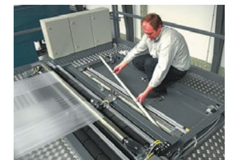
Easy replacement of the sealing and cutting unit. No tools required. Simply open the "Click-lock" and pull out the magnetic sealing unit and replace it with a spare one.
