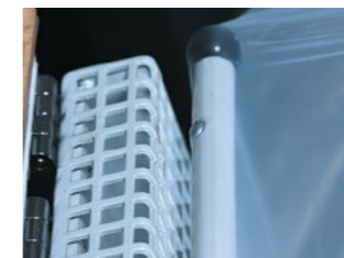
Pneumatic gripper control. Ensures that the film is always placed correctly on the grippers.
