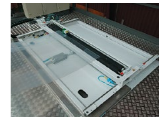
Single film feed device with easy access to the film sealing and cutting unit.
