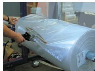
Easy film change at floor level. The end of the old film is simply sealed, taped or stitched to the end of the spare film and automatically fed through the film feed system.
