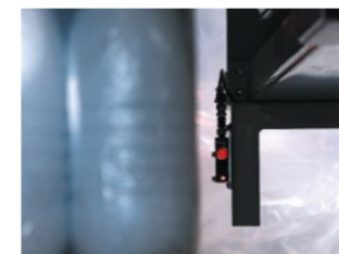
Profile control - the process stops if the photocells are refracted during the downward movement.
